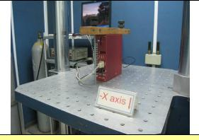
Mechanical Shock Test: +X axis
