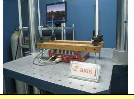
10. Mechanical Shock Test: -Z axis
