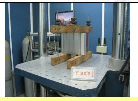
Mechanical Shock Test: -Y axis
