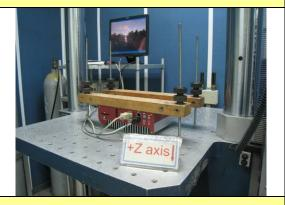
Mechanical Shock Test: +Z axis
