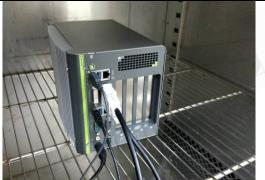
High Temperature/ Humidity Test & Low Temperature Test
